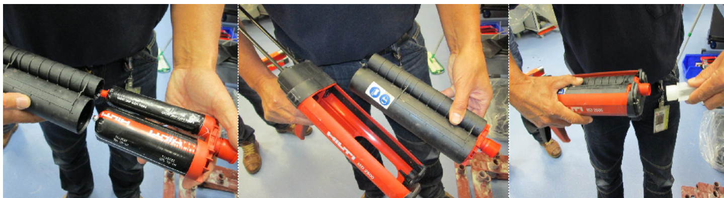
Figure 46: Preparing the mastic gun
